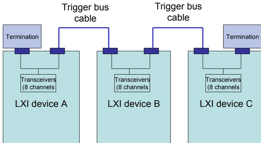
**Figure 1 Connecting three LXI Devices trigger buses together**
