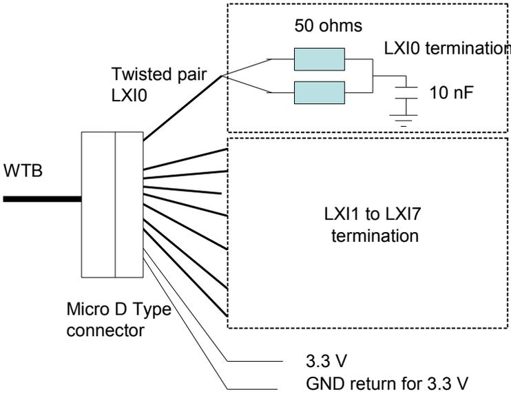
**Figure 2 Schematic representation of a wired bus terminator**
