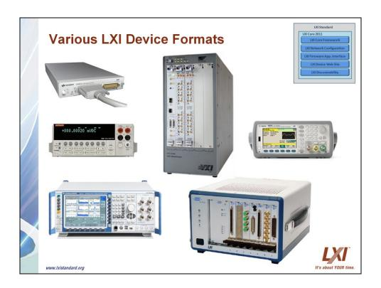
As you can see from the variety of images, an LXI device can take many shapes and forms. Some have elaborate displays and some none at all. Some are card cages with many modules that reveal themselves through the LAN interface both programmatically and via a web page.
