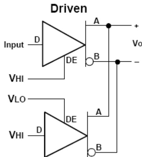
Figure 4 A typical arrangement for the two output drivers in the driven mode of operation
