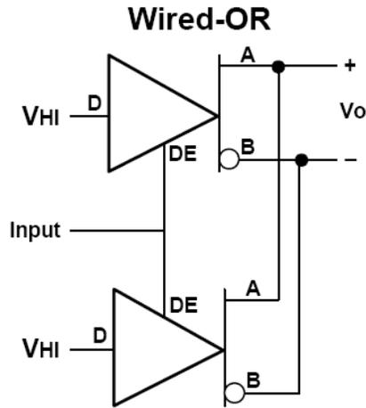
Figure 5 LXI Device trigger bus drivers set to Wired OR mode
