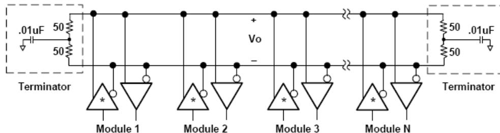
**Figure 3 Representation of a single physical channel of the WTB with transceivers in the LXI Devices driving the bus transmission line**
