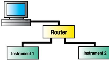
**Description:** Test systems consisting of multiple instruments require a hub, switch or router between the computer and the LXI instrument. This configuration permits the use of regular LAN cables throughout the system.
