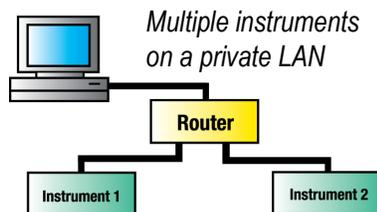
This step-by-step guide emulates configuring multiple instruments on a private LAN using a commercial PC and router. The recommended router utilizes DHCP, which automatically assigns an IP address to an instrument.
