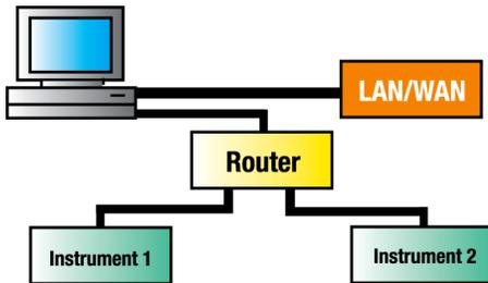
**Description:** Test systems should be isolated from the company network so the test equipment does not share LAN bandwidth with all the other users in the company. This is done effectively by adding a second network interface card (NIC). No intranet/internet user can access the instruments without specific permission.
