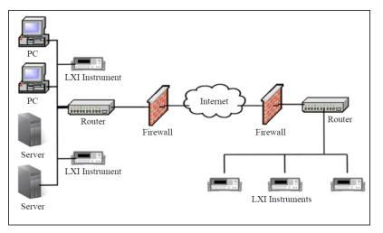
Internet is required, as seen in the figure to the right. Companies with multiple sites already have this method of communication between PCs, and LXI Devices act just like PCs for LAN interconnection.
