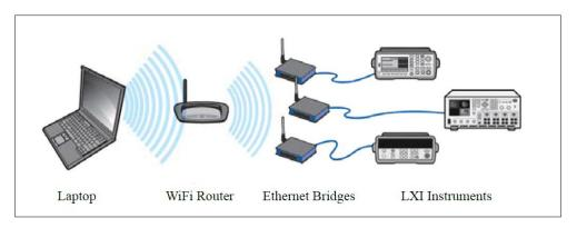
After the device has powered up and a connection to the LAN has been established, an attempt will be made to obtain an IP address as part of its boot-up process. The LXI specification requires every LXI device have a LAN status indicator. Once the connection status is good, this indicates that the LXI device has successfully booted up, obtained an IP address and can be discovered on the network.
