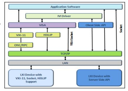
As seen in the figure, test developers can rely solely on the IVI Driver, or they can communicate directly with the LXI Device through multiple interfaces typically available when installing VISA (Virtual Instrument Software Architecture). VISA I/O Libraries come with instrumentation from all vendors of LXI Devices. You can learn more about these interfaces from *Guides For Using LXI Devices*, found at the LXI Consortium site: www.lxistandard.org/About/Default.aspx.
